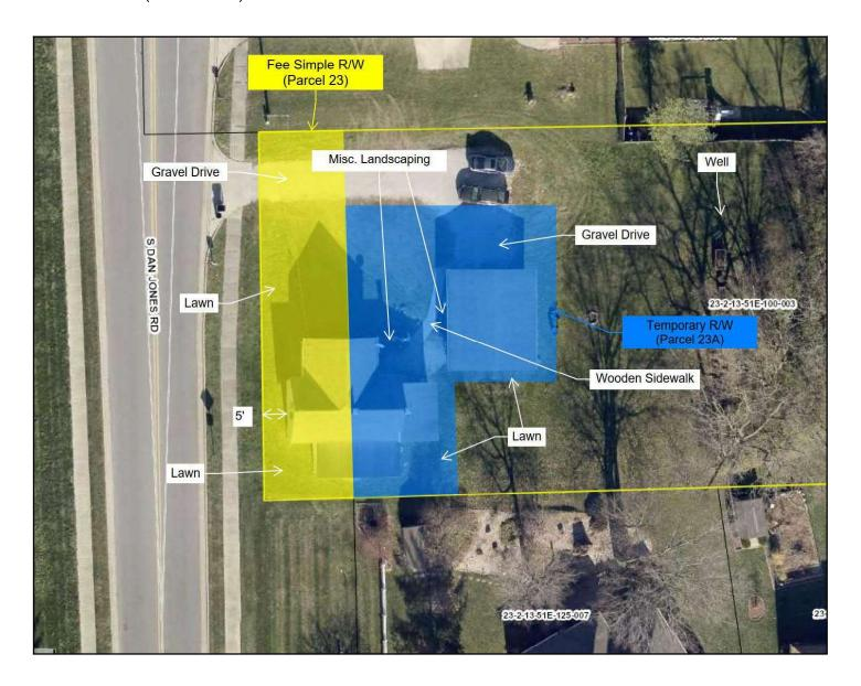
Note: The above sketch was prepared to illustrate the approximate location and physical characteristics of the right of way to be acquired as well as certain physical characteristics of the residue tract. The right-of-way lines were plotted based on the dimensions from the parcel plat and legal descriptions, but their accuracy is not guaranteed. Land improvements not within the vicinity of the acquisition that are unaffected are not labeled.
